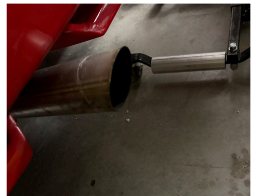
Nice, clear exhaust is good news for the head gasket!
