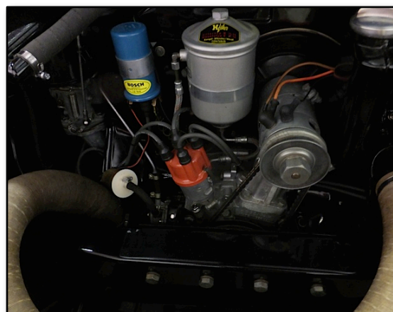
Imaculate 912 engine note the 4 point distributor Photo by Axel Olsen
