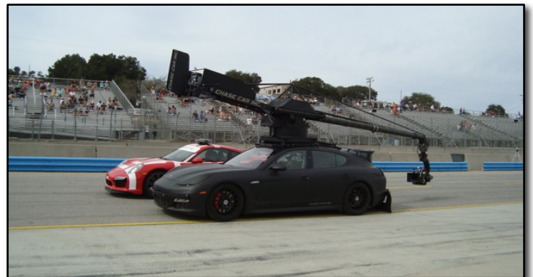
This Panamera Turbo Camera Car has a camera mounted on a movable crane. Cameraman, Jeff Zwart, many-time Pikes Peak winner, operated the camera from a rear mounted turret. Photo by Steve Proctor
